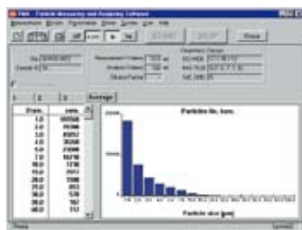
Complete remote control using PAMAS PMA program with data storage in ASCII code.
