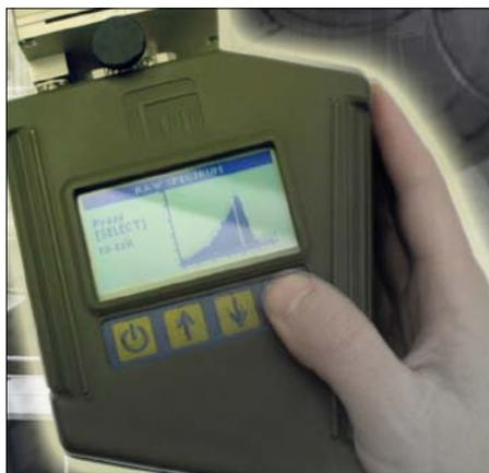
The **FluidScan** is a handheld condition based maintenance system that protects machinery by determining when a lubricant needs to be changed due to excessive contamination or degradation. It detects lubricant contamination and degradation at the point of use by measuring key oil condition parameters in both synthetic and petroleum based lubricants and fluids.
